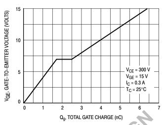
Figure 8. Gate-To-Emitter Voltage versus **Total Charge**
