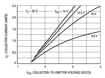
Figure 1. Saturation Characteristics
