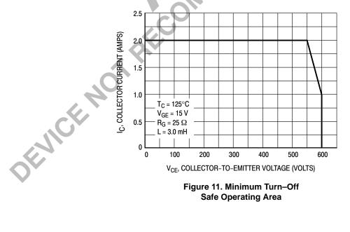
Figure 11. Minimum Turn-Off Safe Operating Area
