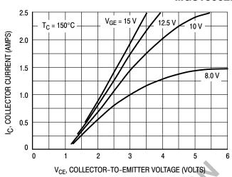
Figure 2. Saturation Characteristics
